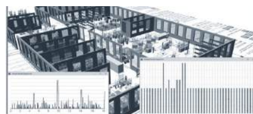
Fig. 2. Simulation based factory planning and optimization (created in Technomatix Plant Simulation)
